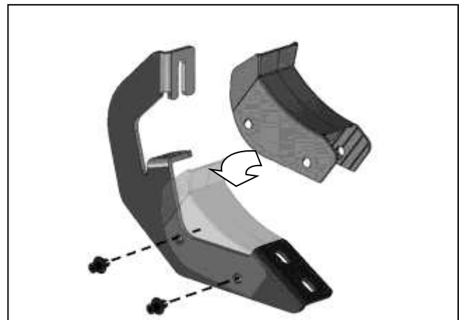
(Fig 8) Slide Cover over top of Bracket. Attach Cover to Bracket with (2) Retaining Clips
