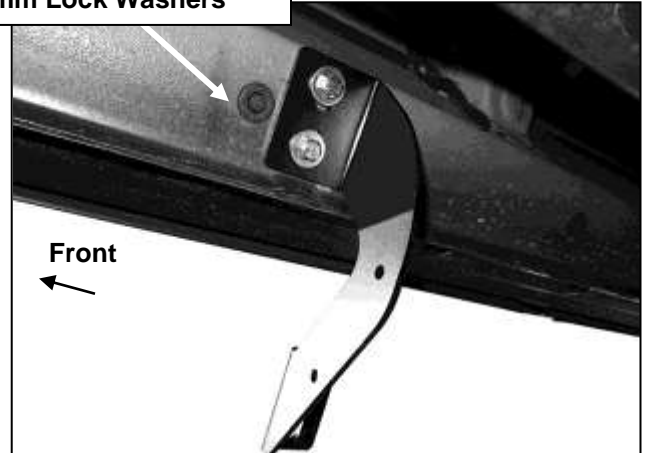
(Fig 7) Passenger side center Bracket installation
